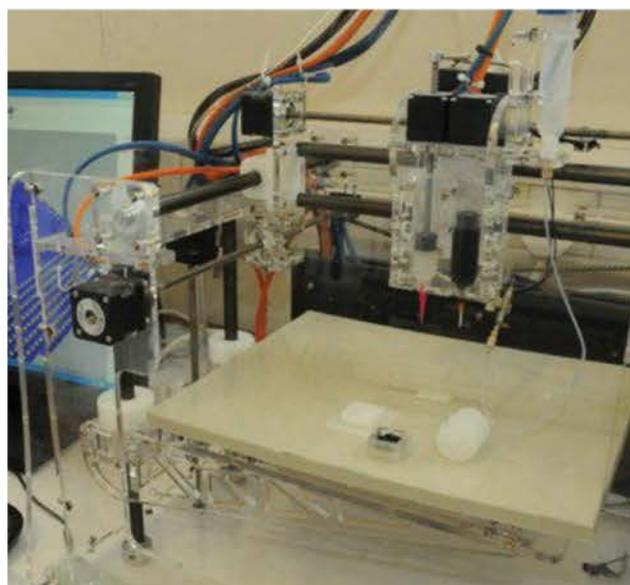
Figure 16-24. Impression de reactionware
